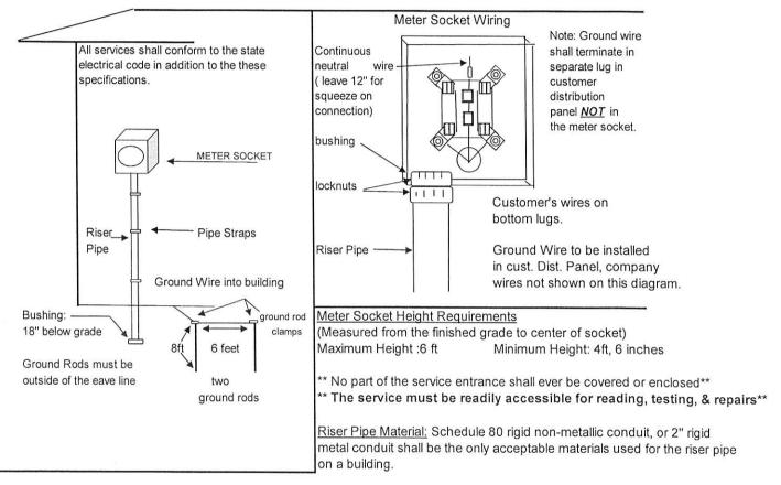
UNDERGROUND SERVICE METER SOCKET MINIMUM SIZE DIMENSION: 200 AMP: 14' X 12" X 4 3/8" SOCKET MUST BE RATED AT 200 AMPS.
