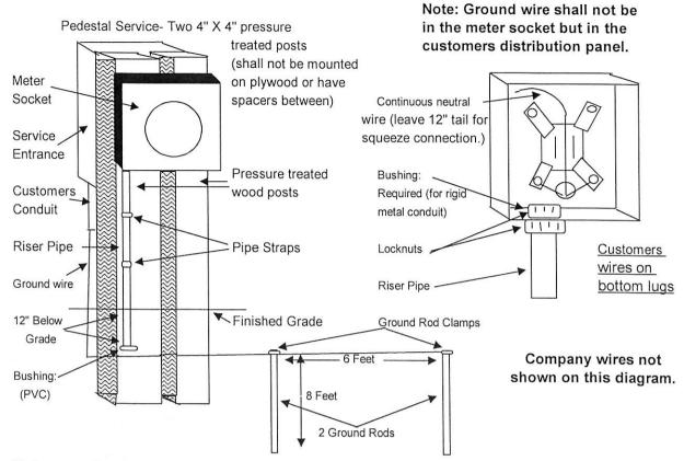
Using an 8' long Post, Approximately 5' shall be above the ground and 3' below ground.
